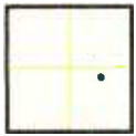
ONE POINT CAPTURED. SINGLE EVENT CAPTURE USING EQUIVALENT TIME SAMPLING. 20 MS/S. 100 MHz DSO.
